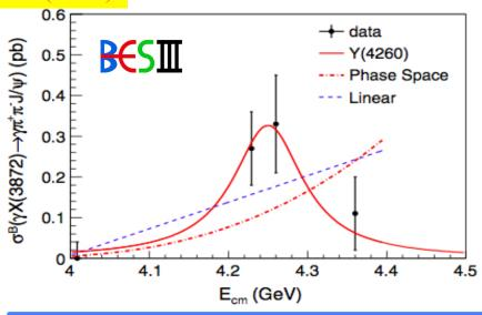
The resonant contribution with Y(4260) line shape provides a better description of the data than either a linear continuum or a E1-transition phase space distribution
