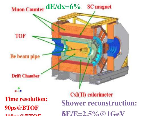
The new BESIII detector is hermetic for neutral and charged particle with excellent resolution, PID, and large coverage.
